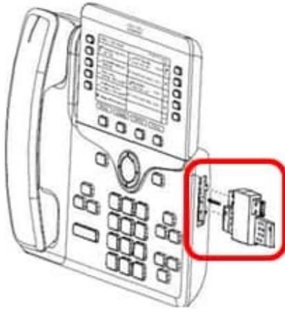
Step 5. Connect the other end of the spine connector to the second KEM.
