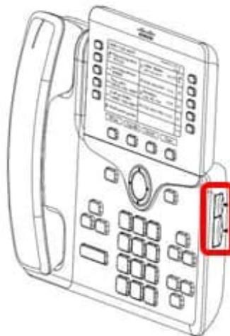
Step 4. Connect one end of the spine connector to the phone.
