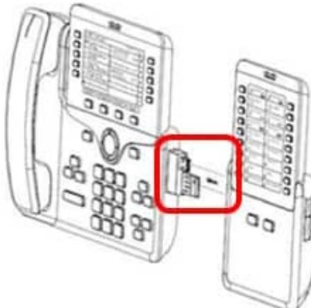
Step 6. Fasten the screws into the slots provided at the phone and the KEM.
