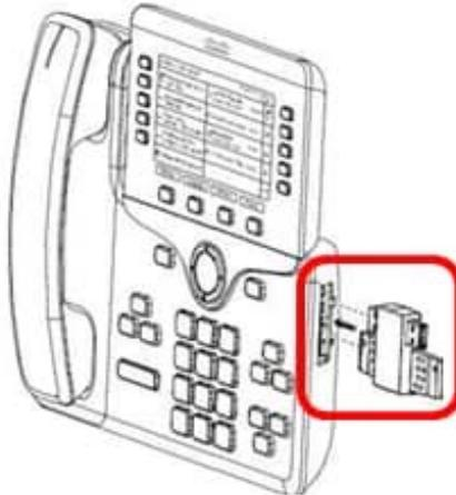
Step 5. Connect the other end of the spine connector to the KEM.
